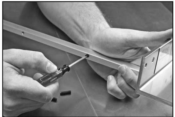
Fine-Tuning Nylon Adjusting Screws.
