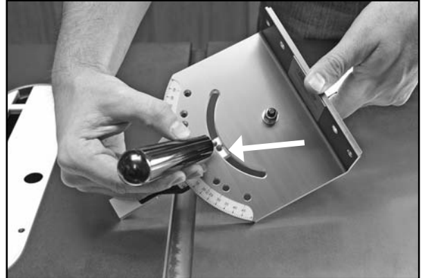
Installing Miter Gauge Handle into Miter Bar.
