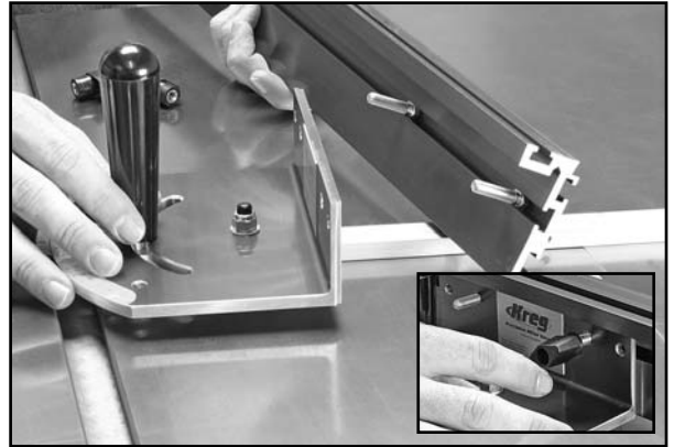
Attaching fence to Miter Gauge Head.
